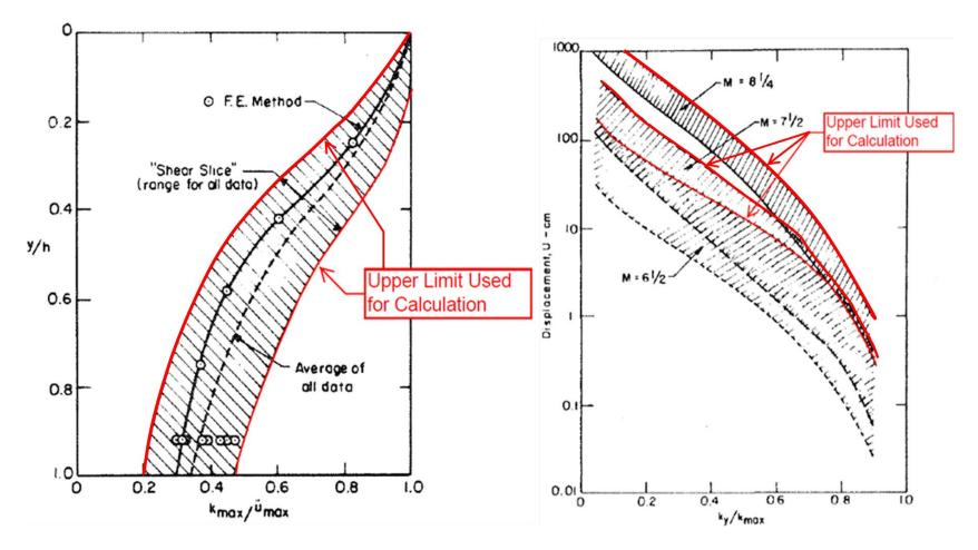
Figure 4-12: a) Variation of "Maximum Acceleration Ratio" with depth of sliding mass; b) Variation of predicted displacement (U) with K<sub>y</sub>/K<sub>max</sub> ratios (Figures from Makdisi and Seed, 1977)
