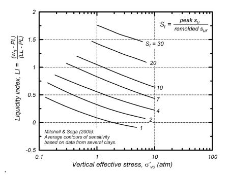
Figure 4-11: Mitchell and Soga (2005) correlations for remolded strength of clays (from Idriss and Boulanger, 2008)
