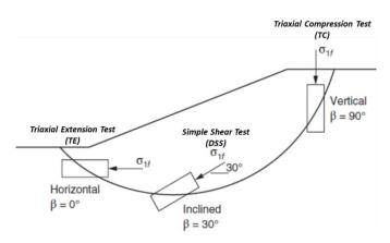
Figure 4-10: Stress orientation at failure and undrained strength anisotropy of clays (Duncan et. al., 2014)
