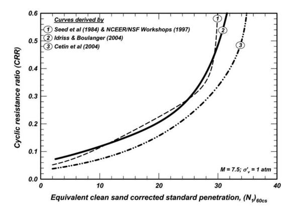
**Figure 4-9: Comparison of SPT-liquefaction triggering correlations** (From Idriss and Boulanger, 2012)
