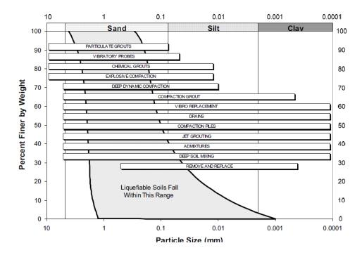
Figure 4-14: General applicability of ground improvement methods for liquefiable soils (from Mitchell, 2008)
