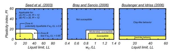
Figure 4-5: Methods used to determine liquefaction susceptibility: Seed et al. (2003); Bray and Sancio (2006); and Boulanger and Idriss (2006).
