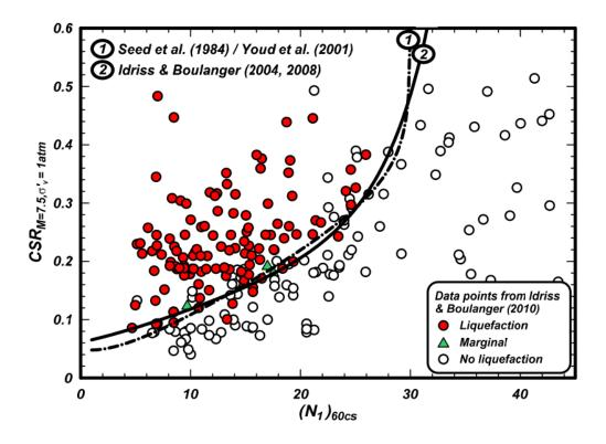
Figure 4-8: Updated database plotted with Idriss and Boulanger 2004 and 2008 SPT-liquefaction triggering correlations (From Boulanger and Idriss, 2014)
