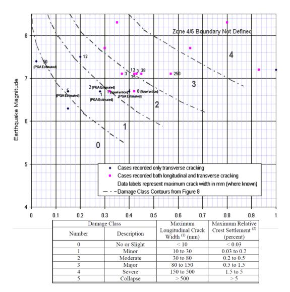
Figure 4-4: Contours of damage class versus earthquake magnitude and peak ground accelerations for earth fill dams (Pells and Fell, 2003)
